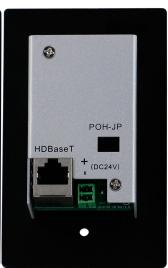
WALL-HDBT-70TR-LITE is an HDBaseT Wallplate transmitter & receiver, it can support 1\*HDMI input, 1\*HDBaseT(RJ45) output. The resolution can up to 4k, with the POC(power over cable) function, users can only power on the HDBaseT receiver. For the transmission distance it can up to 70m at 1080**P 60Hz,1080i 60Hz**, and for 4K, it can up to 40m. It's popularly used in the small meeting room, classroom or other long distance transmission applications.
