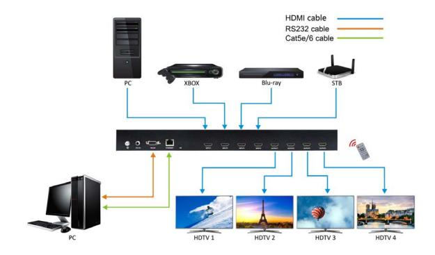
**Application 2: Diagram of Video Wall Displaying**
