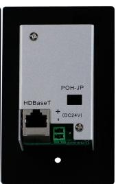
WALL-HDBT-70TR-LITE is an HDBaseT Wallplate transmitter & receiver, it can support 1\*HDMI input, 1\*HDBaseT(RJ45) output. The resolution can up to 4k, with the POC(power over cable) function, users can only power on the HDBaseT receiver. For the transmission distance it can up to 70m at 1080P, and for 4K, it can up to 40m. It's popularly used in the small meeting room, classroom or other long distance transmission applications.
