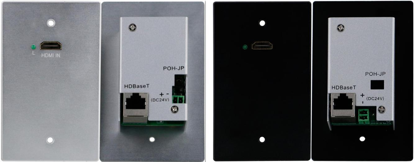
WALL-HDBT-70TR-LITE is an HDBaseT Wallplate transmitter & receiver, it can support 1\*HDMI input, 1\*HDBaseT(RJ45) output. The resolution can up to 4k, with the POC(power over cable) function, users can only power on the HDBaseT receiver. For the transmission distance it can up to 70m at 1080P 60Hz,1080i 60Hz, and for 4K, it can up to 40m. It's popularly used in the small meeting room, classroom or other long distance transmission applications.
