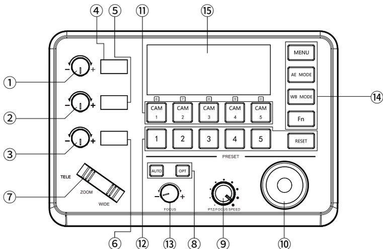
① This Rotation Knob which was to adjustment the Camera Exposure Parameter or Red Gain Value, Turn Right Rotation was to changed the valued Increased, Turn Left Rotation was changed the Valued Decreased.
